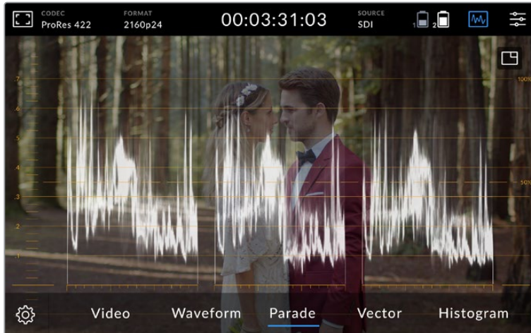
The RGB parade displays separate waveforms displaying the luminance of the red, green and blue channels
